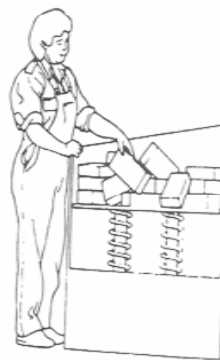
After Self-levelling work surface
